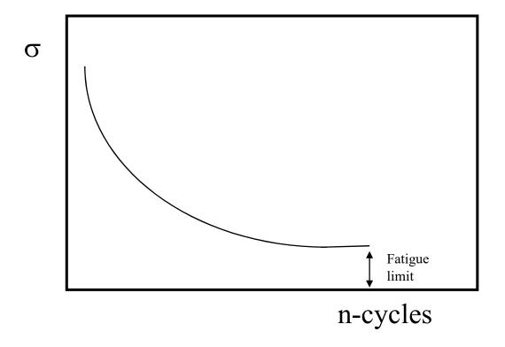
It is difficult (or impossible) to accurately predict the actual fatigue limit for a given part. The only sure way is to test to failure.
